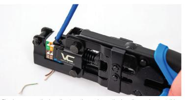
Firmly squeeze the handles together, release the handles and repeat this step to ensure a proper termination.
