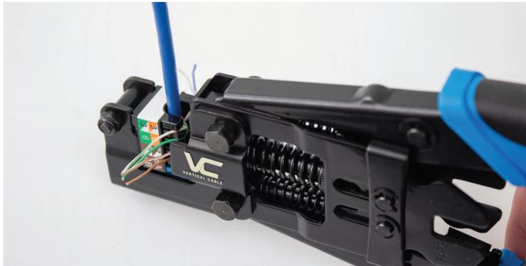
Insert prepared jack & cable assembly into the I-Punch Tool.
