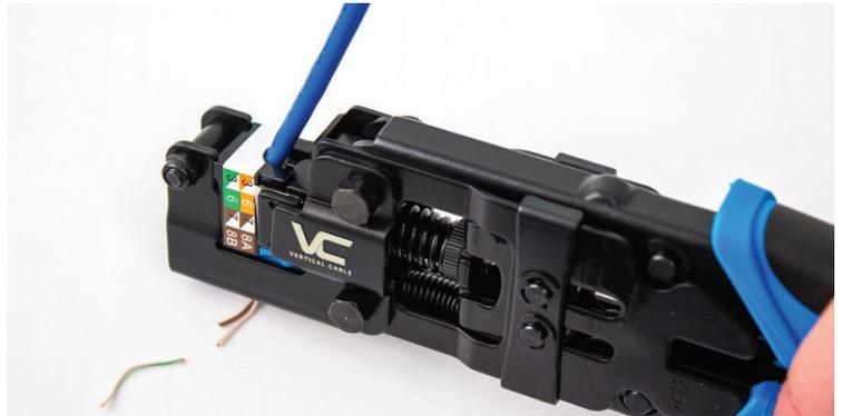
Firmly squeeze the handles together, release the handles and repeat this step to ensure a proper termination.
