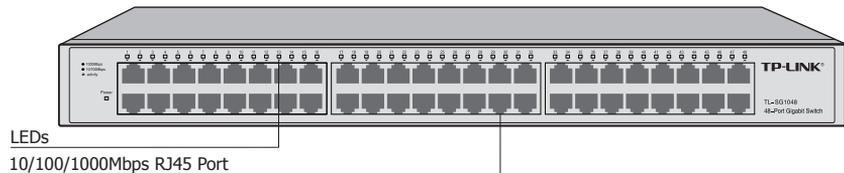
Figure 1-1 Front Panel of TL-SG1048
