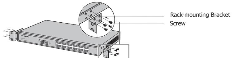
Figure 2-2 Bracket Installation
