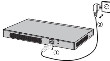
Figure 4-2 Connecting to Power Supply
