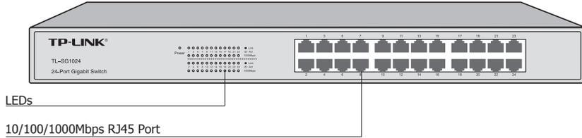
Figure 1-2 Front Panel of TL-SG1024
