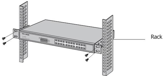
Figure 2-3 Rack Installation
