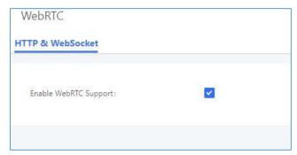
Figure 154: Enabling WebRTC Feature
