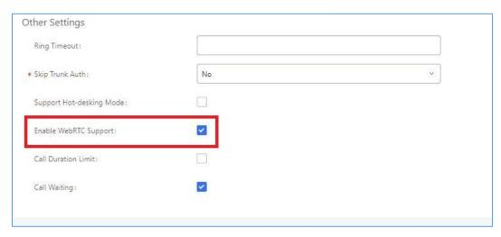
Figure 155: Enabling WebRTC on Extensions
