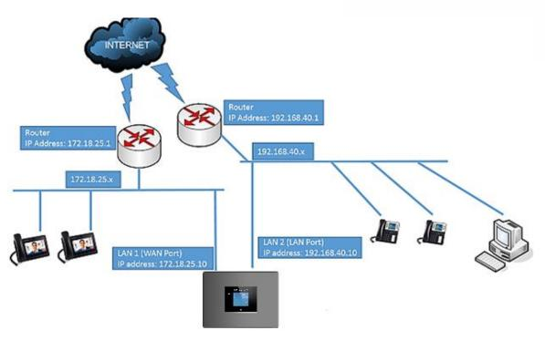
Figure 18: UCM6302 Network Interface Method: Dual
