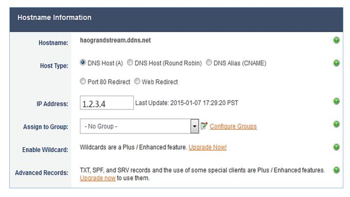
Figure 27: Register Domain Name on noip.com
