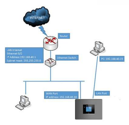
Figure 17: UCM6302 Network Interface Method: Switch
