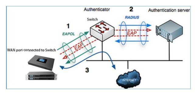
Figure 19: UCM630X Using 802.1X as Client
