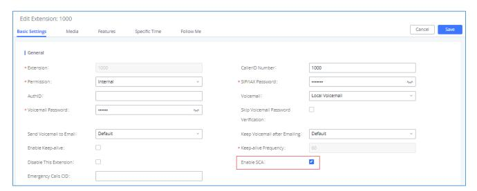
Figure 226: Enabling SCA option under Extension's Settings
