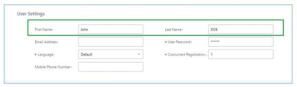
Figure 211: Configure Extension First Name and Last Name
