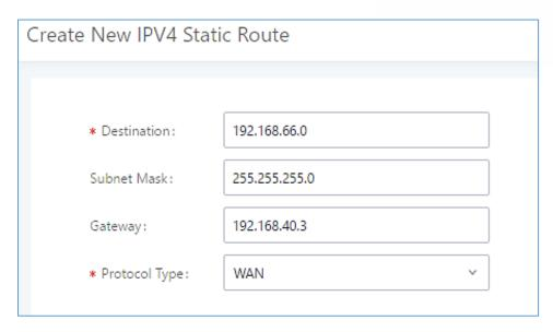
Figure 22: UCM6304 Static Route Configuration
