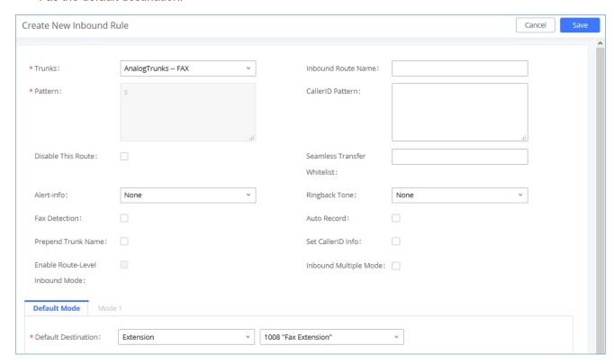
Figure 131: Configure Inbound Rule for Fax
