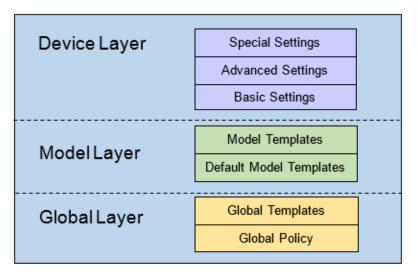
Figure 55: Zero Config Configuration Architecture for End Point Device
