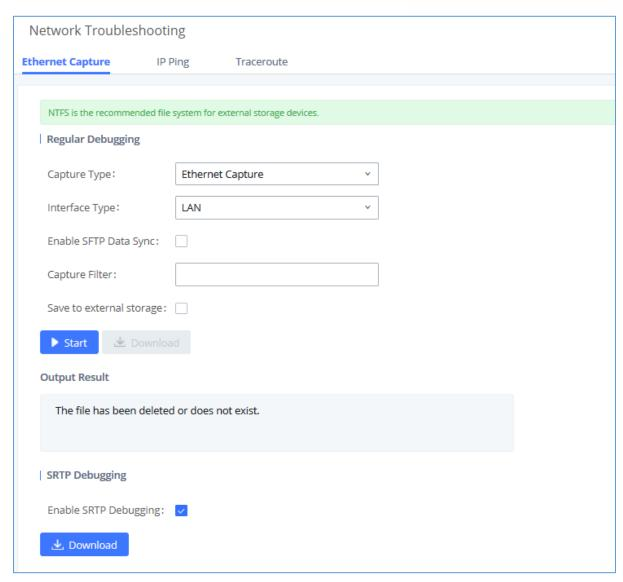
Figure 339: Ethernet Capture
