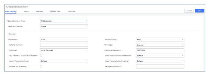
Figure 129: Configure Extension for Fax Machine: FXS Extension
