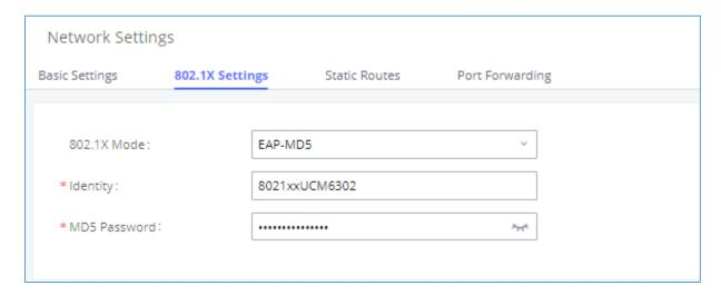
Figure 20: UCM630X Using 802.1X EAP-MD5
