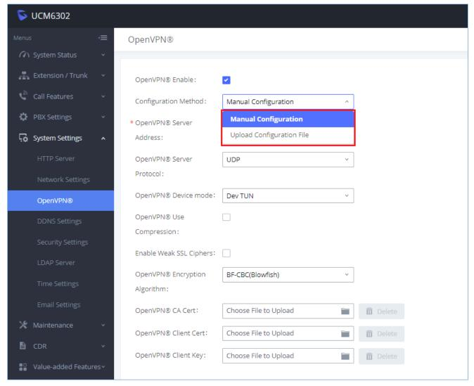
Figure 26: Open VPN® Feature on the UCM630X
