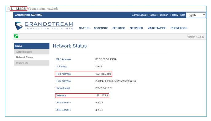
Figure 25: GXP2160 Web Access using UCM6302 Port Forwarding
