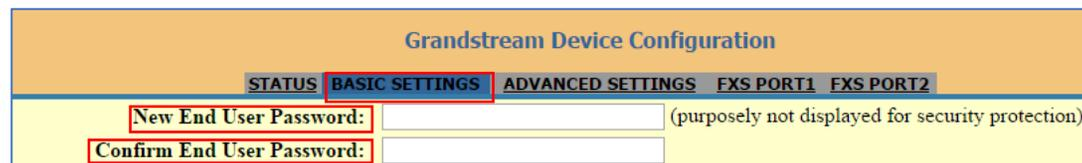
The screenshot shows the 'Grandstream Device Configuration' web interface. At the top, there is a navigation bar with tabs: STATUS, **BASIC SETTINGS**, ADVANCED SETTINGS, FXS PORT1, and FXS PORT2. Below the navigation bar, there are two input fields: 'New End User Password:' and 'Confirm End User Password:'. The 'New End User Password:' field has a note '(purposely not displayed for security protection)' to its right. The 'Confirm End User Password:' field is empty.
