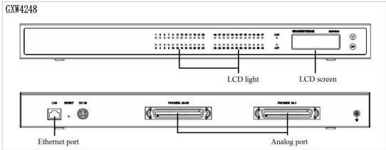
Figure 1: Diagram of GXW4216/24/32/48 Panel
