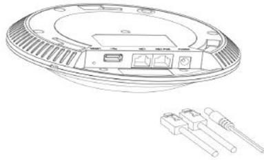
Figure 8: Connecting GWN AP - GWN7600 as example
