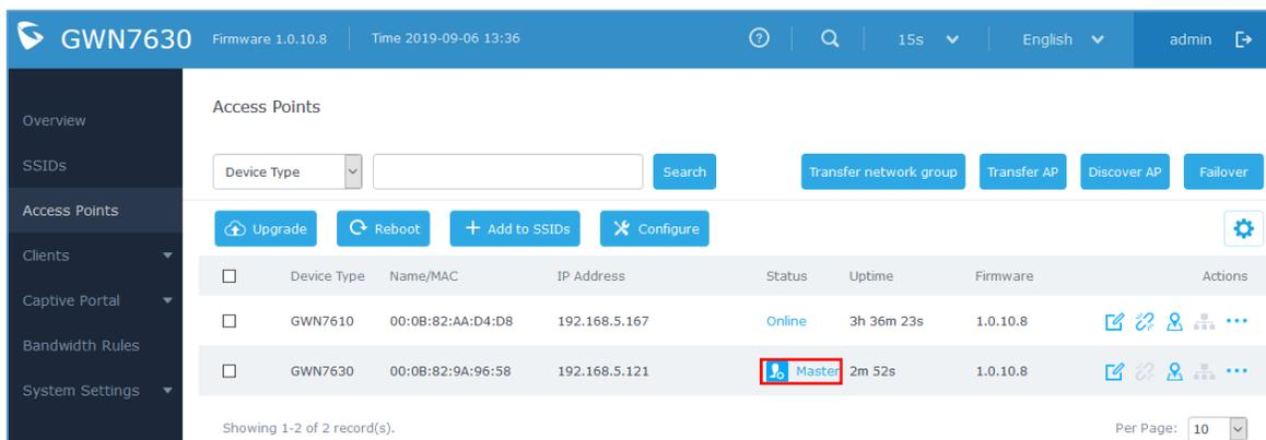
**Figure 45: Then new assigned Master AP web interface**
