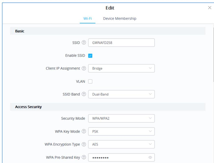
**Figure 65: Add a new SSID**
